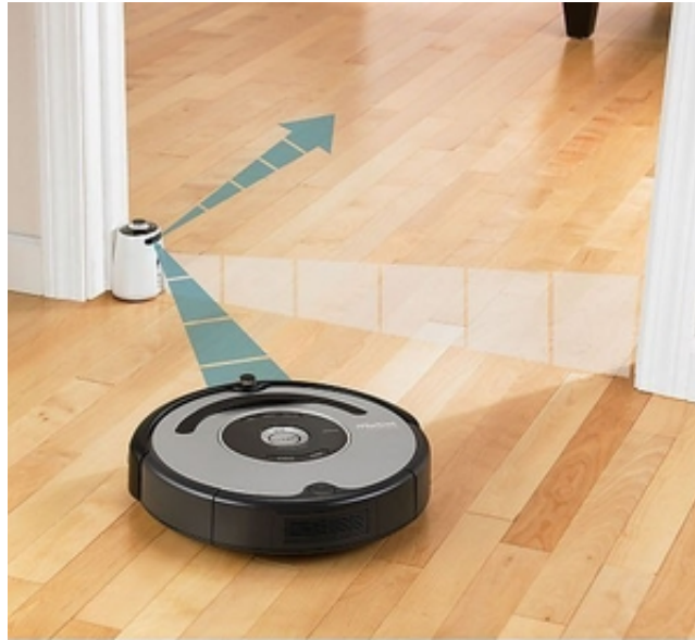
A Virtual Wall Lighthouse directs Roomba to clean one room entirely before moving to the next and creates an invisible barrier.
